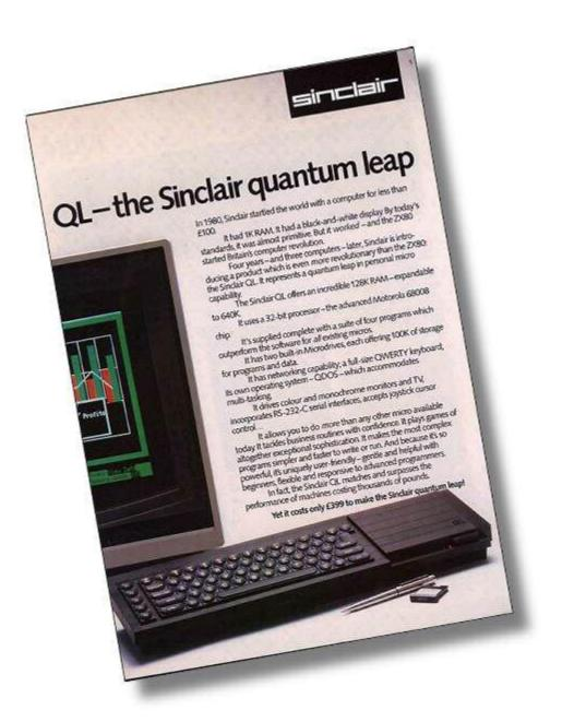
promising, with a 32 bit processor running at 7.5Mhz and operating system support for multitasking and windows. It was to have a proper full-travel keyboard along with 128Kb of RAM, basic networking and RS232 communications. There was also a bundled office suite written by Psion Software comprising Quill
