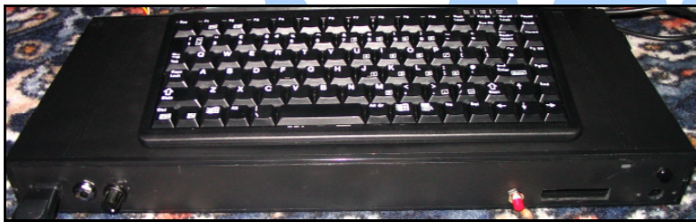
Above: The ZXSE prototype in a rack-mount case, using a Cherry keyboard with Kempston joystick, headphones, volume, NMI, dual CF slot, LED and PS/2 slots visible.
