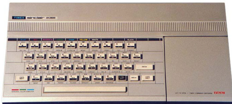
Above: The Timex-Sinclair 2068 (I have no idea why that number) was an officially licensed Spectrum 'clone'. Software could be loaded via cartridges (see bottom) that were plugged in under that panel on the right. Below: Not much is known about the Diagra except that it's a Russian and by a company called Dynamo Computer. For what it's worth, I think it looks just fantastic (and it's probably more Spectrum compatible than the TS2068. All images this page sourced from Planet Sinclair .
